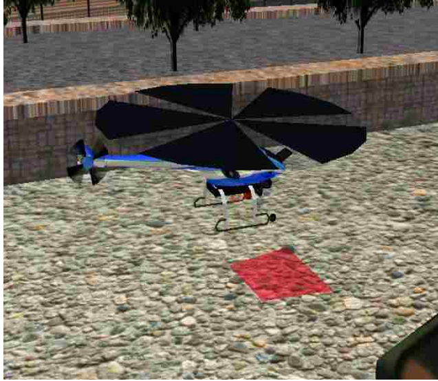
Figure 1.1: A typical PALACE landing starts at 30 m AGL and proceeds downward in 6 m increments. Navigation by machine vision operates from 12 m to 2 m AGL.
