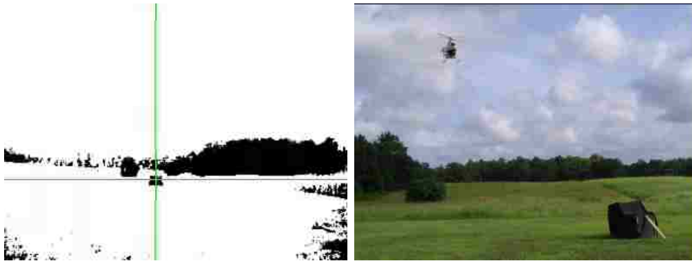
Figure 1.7: The Georgia Tech rotorcraft UAV tracks a target to hold a position.
